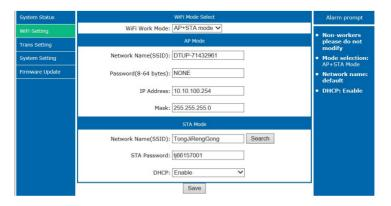
4. Click the search button in the lower right corner, select the Wi-Fi name to be connected to the monitoring device.
